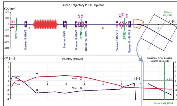
Figure 4: TTF injector trajectory simulation.
