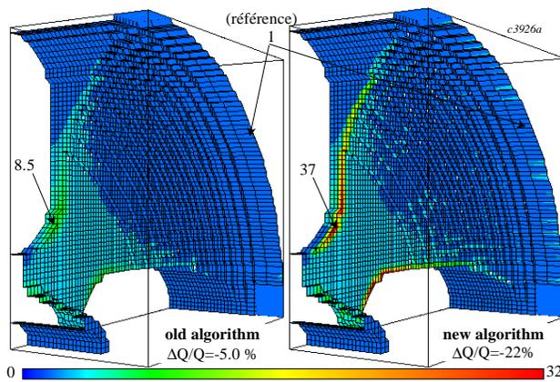
Fig. 7. Losses in the Trispal cavity ( $\pi$ -mode).
