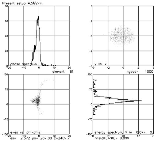
Figure 3: Various distributions of the longitudinal phase space at the entrance to the main cryomodule.
