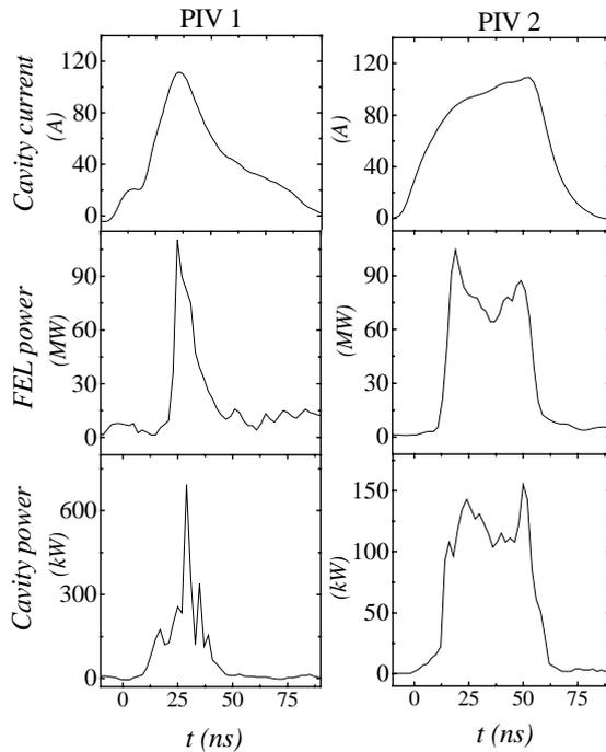
Figure 4 : Cavity output current, FEL output power and High-Q cavity output power in PIV-1 and PIV-2.
