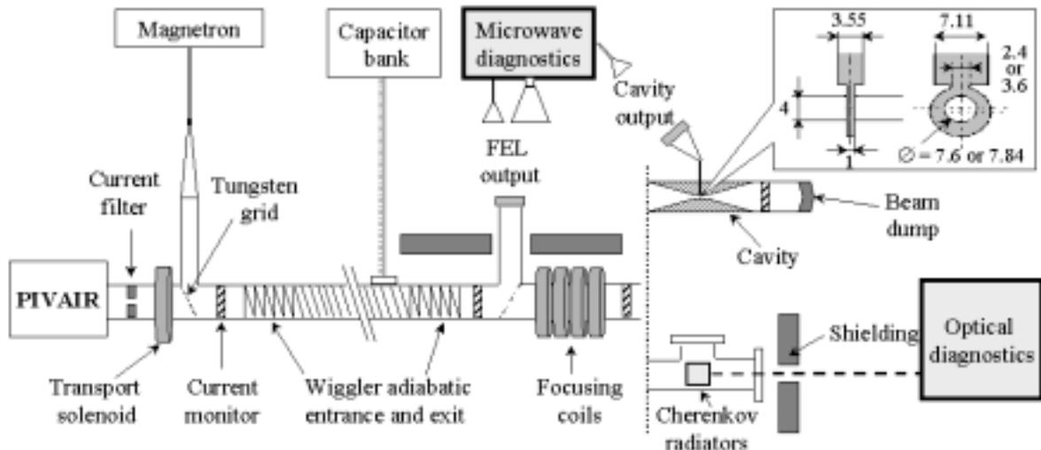
Figure 3 : PIVAIR Experimental Set-Up
