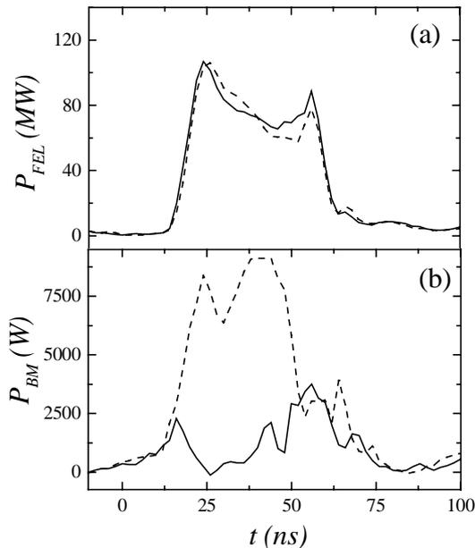
Figure 2 : Reproducibility of the FEL power signal and the sensitivity of the bunch monitor power.
