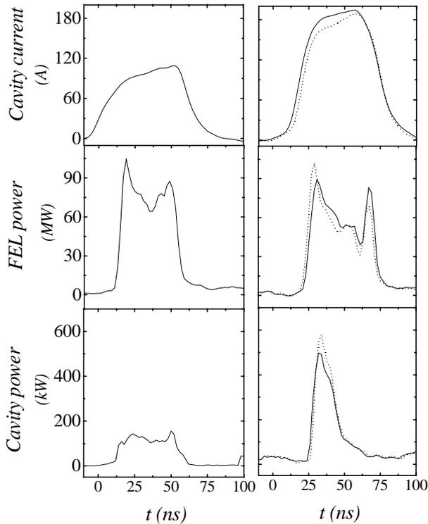
Figure 4 : Cavity output current, FEL output power and high-Q cavity output power for two different focusing configurations
