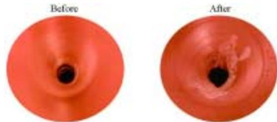
Figure 3 : Two photographs representing the low-Q cavity entrance , before and after beam heating.
