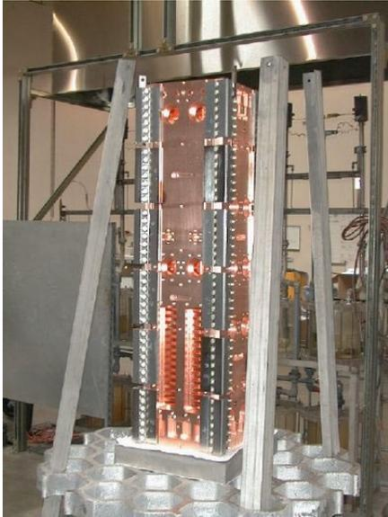
Figure 2 - The RFQ module ready for the final braze
