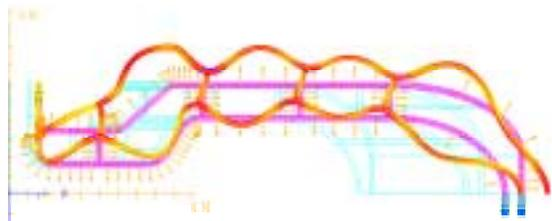
Fig. 4. Mechanical deformation as a result of 1 bar pressure increase in the helium bath. The maximum displacement is about 20  $\mu\text{m}$  in the outer shell (for clarity, the deformation is amplified in the picture).
