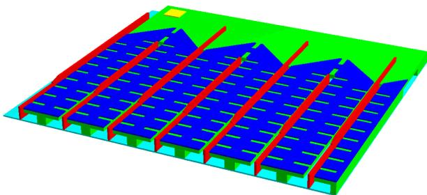
Figure 2: A part of the MAFIA model: notched metal meander strip (dark-blue) on dielectric supports (green), metal separators (red) are connected to the ground plate (light-blue, below). Compare Fig. 1.
