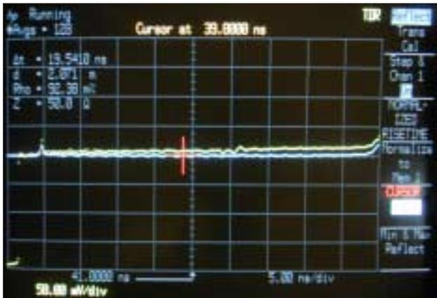
Figure 4: TDR reflection measurements.
