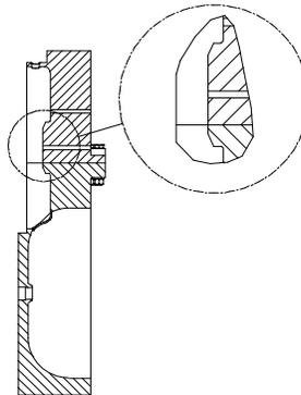
Figure 5. Chamfered CC Posts for Reduced Sensitivity.
