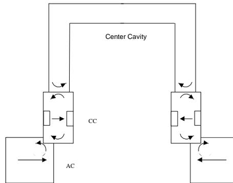
Figure 2. Field Pattern Inside Bridge Coupled Model.
