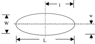
Fig. 6. Definition of Full and Half, Lengths and Widths.
