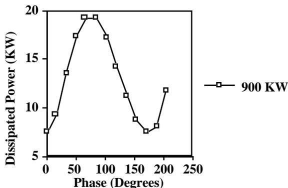
Figure 3: Plot of Dissipated Power versus Phase for the AFT 700 MHz Circulator Tested at LANL.
