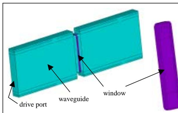
Figure 1, RF window/waveguide model dielectric constant and its loss tangent.
