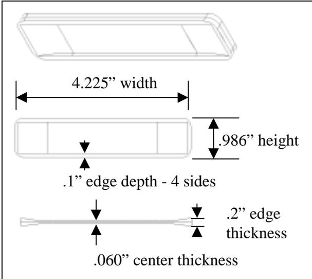
Figure 2, Window design parameters
