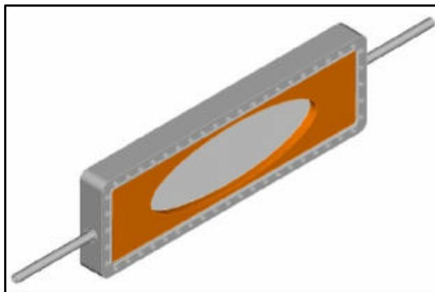
Figure 8: Complete CESR Window Assembly
