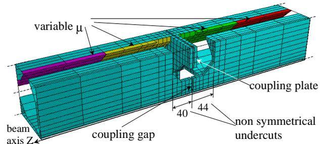
Fig. 5. Resonant coupling (as simulated in section 5).
