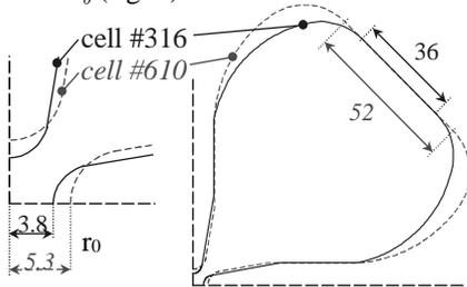
Fig. 1. RFQ cross-sections at two different locations.
