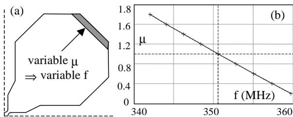
Fig. 6. Simulating  $\Delta f$  with a variable  $\mu$  zone.
