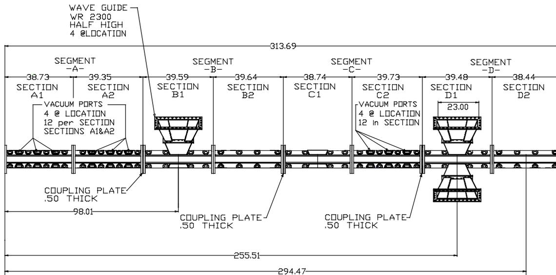
Figure 1: Line drawing of 8-m-long RFQ. This drawing shows the six RF-waveguide feeds used to power the RFQ; two on Section B1 and four on section D1.
