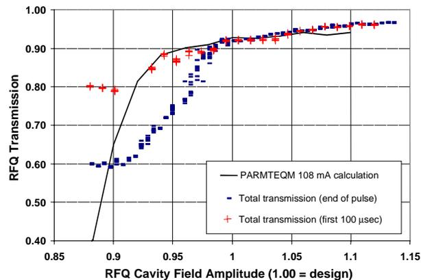
Figure 3: RFQ transmission versus cavity field using a 300- $\mu$ s-long-beam pulse. The anomalous transmission drop occurs at slightly higher fields for longer pulses and CW beams. The calculated transmission is for accelerated beam only.
