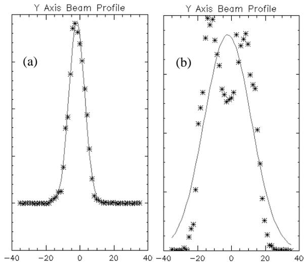
Figure 5: Two vertical wire-scan measurements [19] of beam profile; (a) during the first half, and (b) during last half of beam pulses similar to that shown in figure 4. The HEBT setting was for a Y-emittance scan (near the minimum width in Y) [15] for (a) and (b). The curves are Gaussian fits the data (\*).
