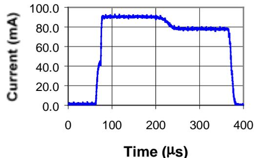
Figure 4: RFQ output beam current vs. time for a 300- $\mu$ s-long pulse at  $\sim 97\%$  of the design RF-field level.
