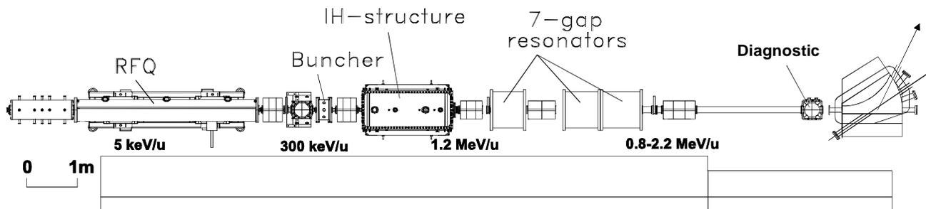
Figure 1: Lay-out of the REX-ISOLDE linear accelerator
