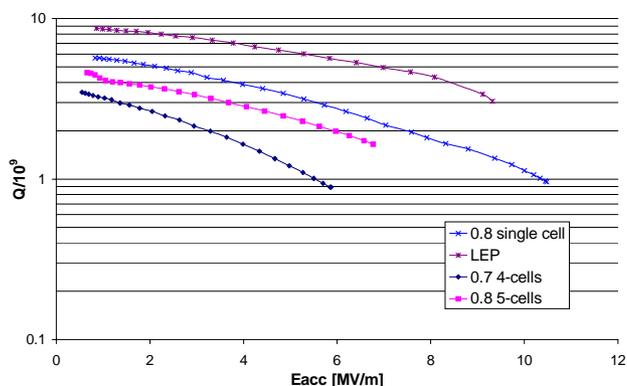
Figure 6: Q vs. gradient of the sputtered-Nb cavities
