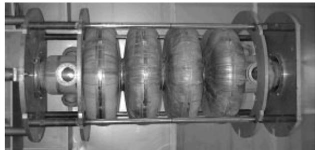
Figure 5: The prototype 4-cell  $\beta=0.7$  cavity
