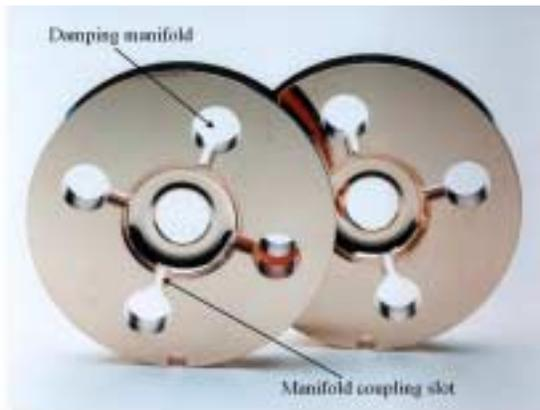
Figure 1: Two cells of NLC Structure RDDS1.
