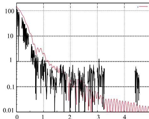
Figure 4: Plot of the measured and computed (smooth) transverse wakefields,  $V/(pC \cdot mm)$  vs. nanosec.
