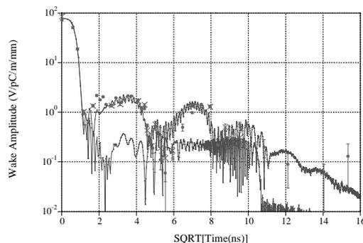
Figure 7: ASSET wakefield data (vertical = dots, horizontal = crosses) and prediction with and without central frequency errors.
