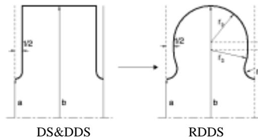
Figure 2: Cell shapes for different disc loaded waveguides.
