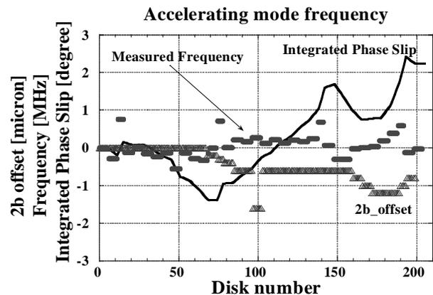
Figure 6: Fundamental mode measurement from stack QC.
