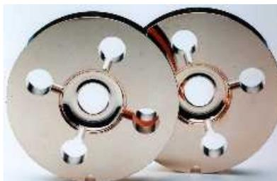
Figure 1. Round damped-detuned structure: cell profile optimized for rf efficiency, dipole modes detuned and damped to suppress long-range wakefield.
