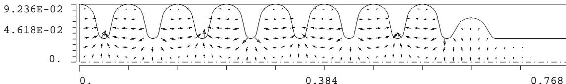
Figure 6: Right half of the transverse mode cavity. The electric field of the 1.95 GHz  $\pi$ -dipole-mode is shown (MAFIA calculation [6]). 15 cells contribute to the deflection, while the end-cells match the field to that in the beam pipe.
