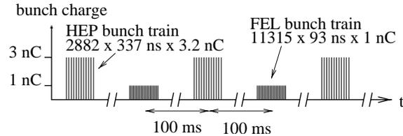
Figure 2: HEP and FEL beam pulse structure
