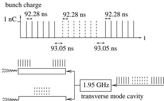
Figure 4: Principle of a fast FEL-Beam switchyard
