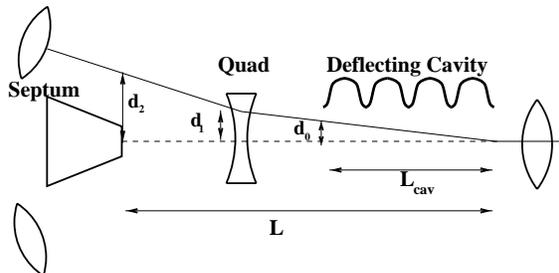
Figure 5: Fast FEL-Beam Splitter. The kick due to the deflecting mode is enhanced by a defocusing quadrupole magnet.
