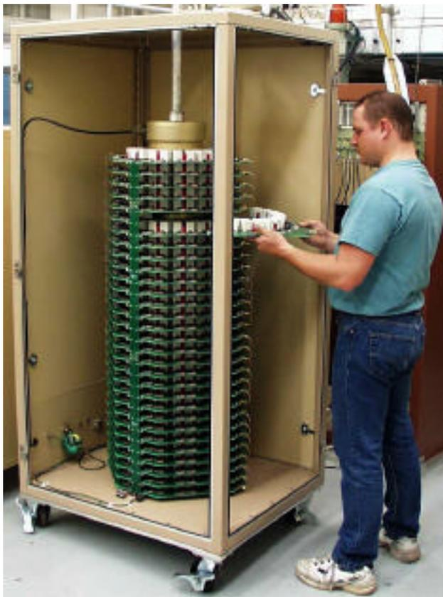
Fig. 5 Complete Kicker Modulator Assembly
