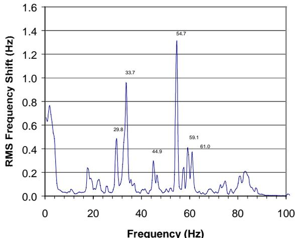
Figure 2. Actual 7-cell cavity microphonics baseline.
