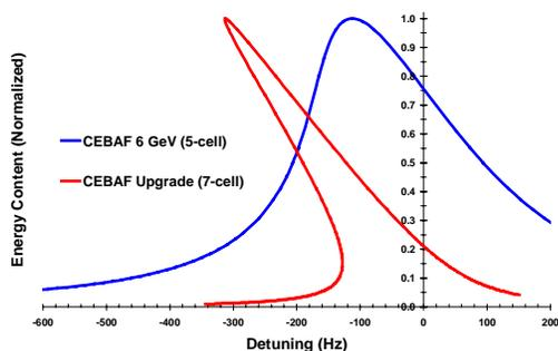
Figure 3. Resonance curves for a typical 5-cell cavity operating in CEBAF at 7.5 MV/m and  $Q_{\text{ext}}$  of  $5 \times 10^6$  and for the 7-cell upgrade cavity at design gradient of 12.5 MV/m and  $Q_{\text{ext}}$  of  $2.2 \times 10^7$ .
