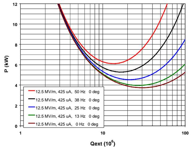
Figure 1. Forward RF power as a function of  $Q_{\text{ext}}$  at the design operating parameters of the 7-cell cavity for several amount of detuning.
