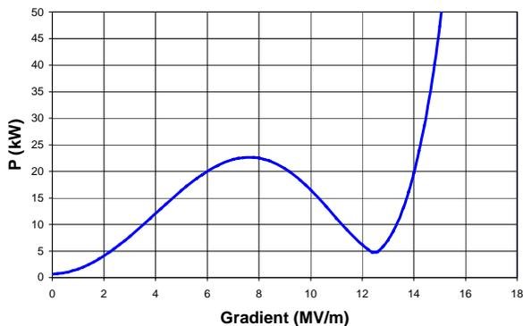
Figure 4. RF power as a function of gradient for the design parameters of the 7-cell cavity. The cavity frequency has been tuned so the cavity will be on resonance at operating field.
