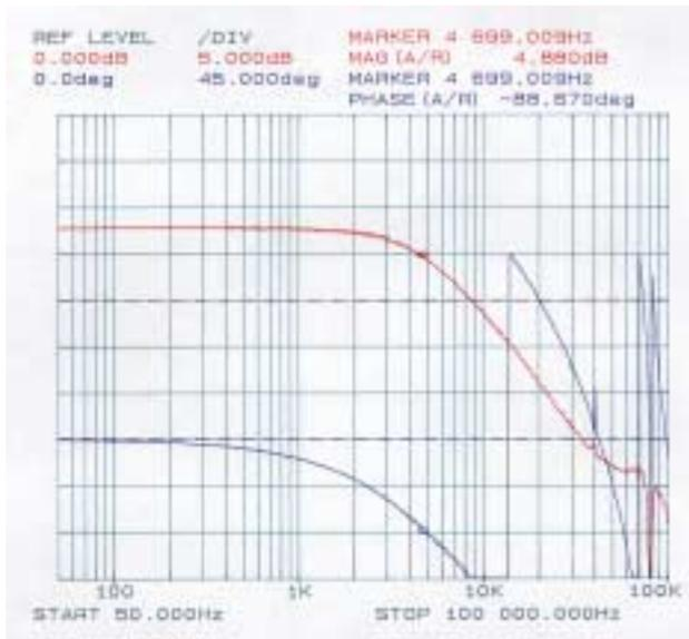
Figure 4: Measured frequency response of FCM with just digital (integrator) control.
