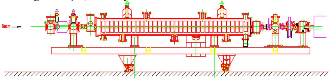
Figure 1: The girder with the MEBT (left), RFQ tank (centre) and LEBT (right)
