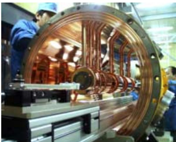
Figure 2: The prototype of the DTL for the high-power test.
