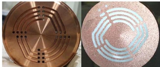
Fig. 2a: Groove processing for the water-cooling channel.
