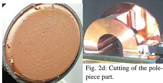
Fig. 2c: PR electroformed surface.
