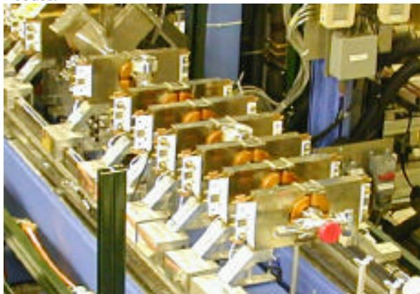
Fig 2. First 7 of the 52 quadrupole magnets in a 11-m section of beamline following the LEDA RFQ.
