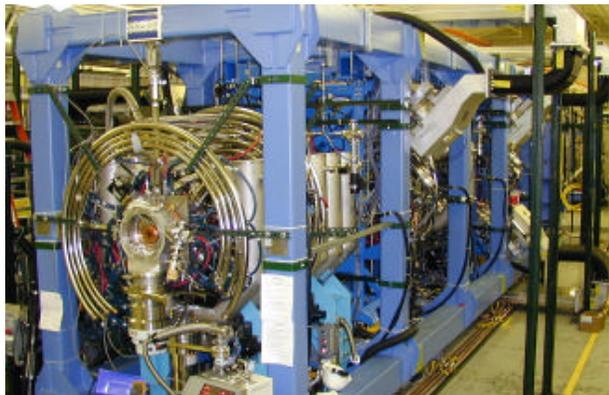
Fig 1. LEDA RFQ mounted in its support frame.
