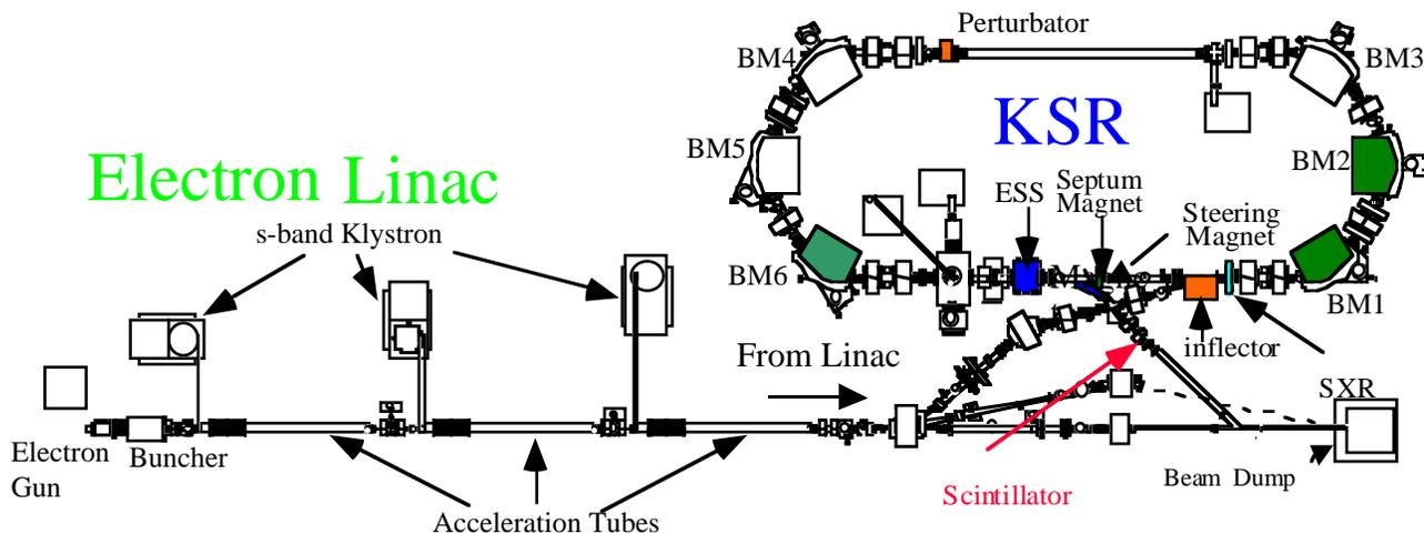
Fig.1 Layout of the 100 MeV electron linac and its pulse stretcher, KSR.
