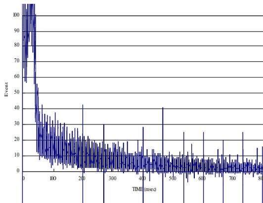
Fig. 8 Count rate of the scintillator in 100  $\mu$ sec time interval during 800 msec.
