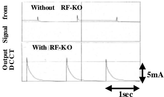
Fig. 7. Circulating beam signal observed by a DCCT without (upper) and with (lower) RFKO.
