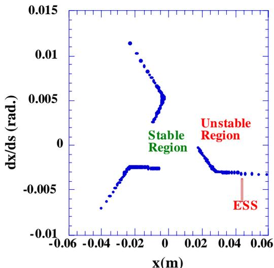
Fig.2 Separatrix (boundary of the stable and unstable regions) in the transverse phase space
