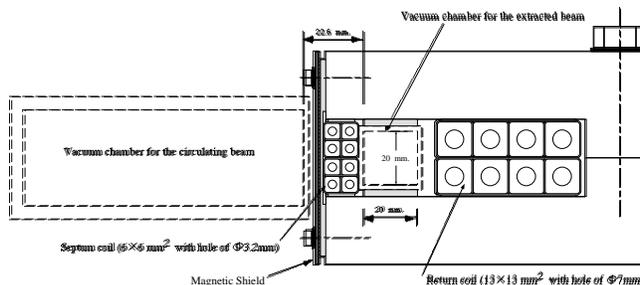
Fig.5 Cross-sectional view of the septum magnet.
