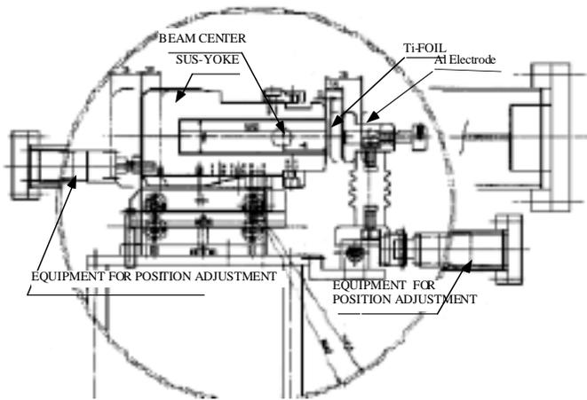
Fig.3 Cross-sectional view of the Electrostatic Septum (ESS).
