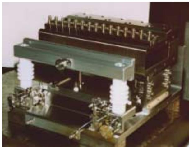
Fig. 4 Overall view of the electrostatic septum before installation into the vacuum vessel.
