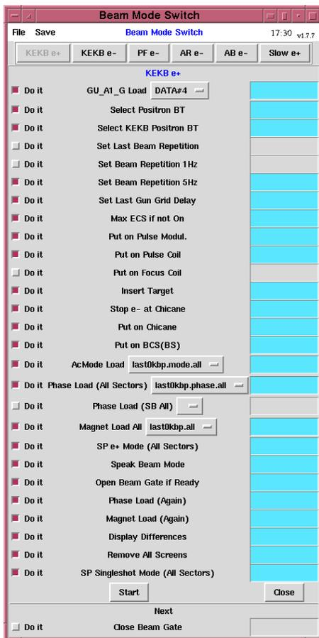
Figure 1: An example of the linac beam mode switch panel. In this example, KEKB  $e^+$  injection was selected. The check-buttons on the left are used to select items to go through. Pull-down-menus are used to choose parameter files. The boxes on the right show the execution status.
