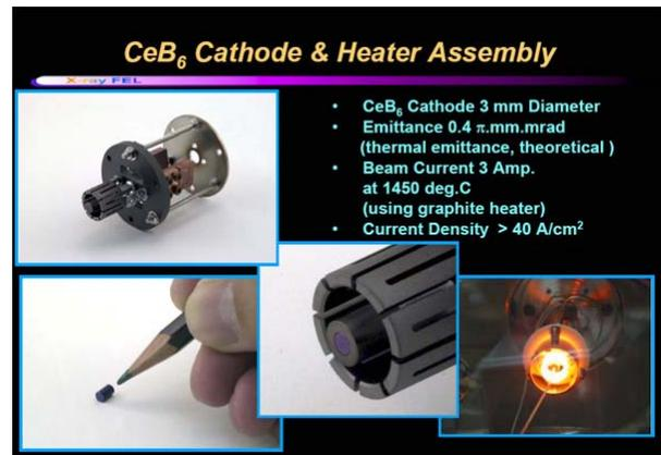
Fig. 3 CeB<sub>6</sub> single crystal thermionic cathode for low emittance electron source.
