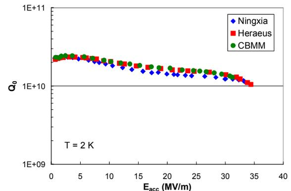
Figure 5: Performance of 1.3 GHz TESLA single-cells made of large grain niobium [6].
