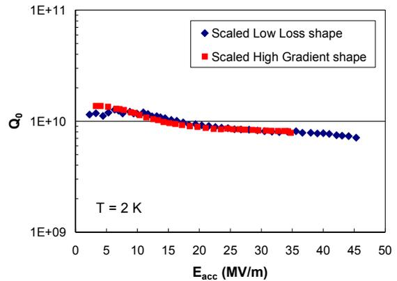
Figure 4: Performance of 2.3 GHz single-cells made of single-crystal niobium. The limitation was quench at  $B_p = 150$  mT in the scaled High Gradient shape cavity and at  $B_p = 160$  mT in the scaled Low Loss shape cavity [5].
