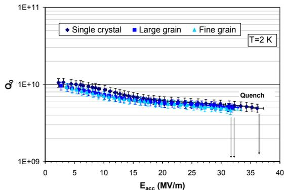
Figure 6:  $Q_0$  vs.  $E_{acc}$  for single-cell cavities with the same shape made of niobium with different grain size [8].
