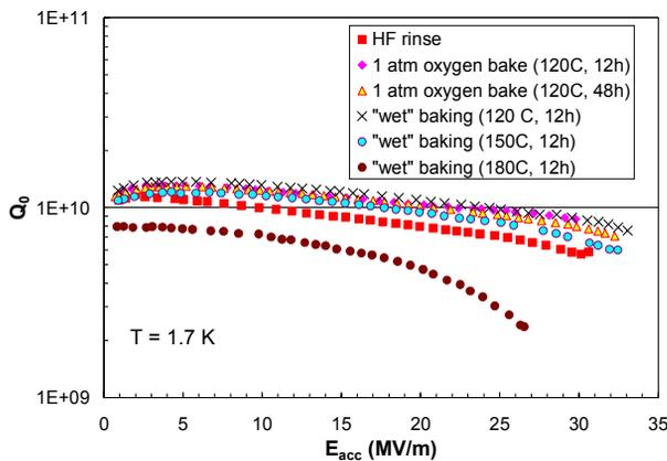
Figure 10:  $Q_0$  vs.  $E_{acc}$  for a 1.5 GHz large-grain cavity of the CEBAF shape after various bakes. The treatments shown in the legend were done sequentially in time after the 2<sup>nd</sup> UHV baking shown in Fig. 7.
