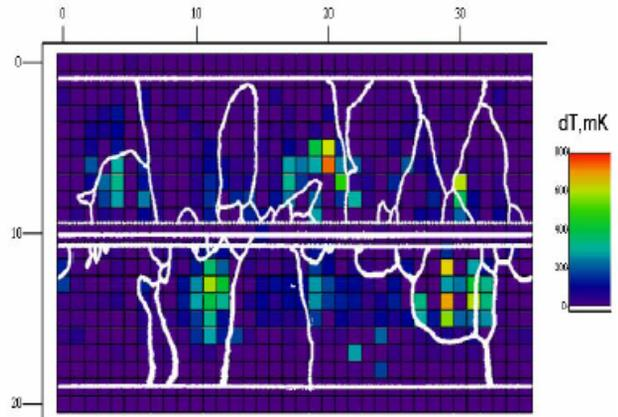
Figure 8: Temperature map in the Q-drop region of a large grain single-cell. The white lines show the grain boundary location [12].
