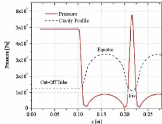
Figure 11: Water pressure variation on the cavity wall along the axis for a TESLA cavity [21].
