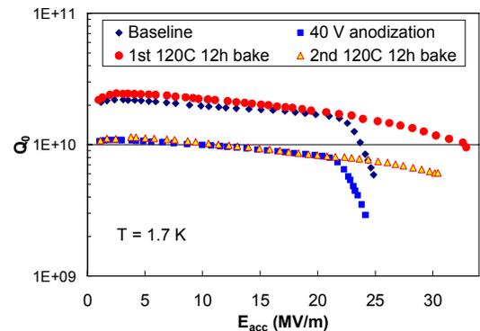
Figure 7:  $Q_0$  vs.  $E_{acc}$  for a 1.5 GHz large-grain cavity of the CEBAF shape showing the re-occurrence of the Q-drop after anodizing at 40 V.
