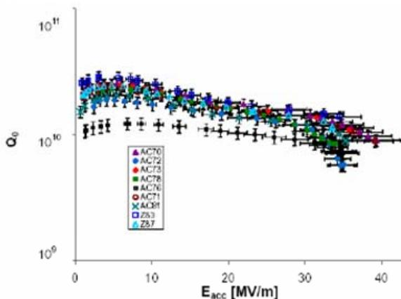
Figure 3: Best performances of 9-cell TESLA cavities [3].
