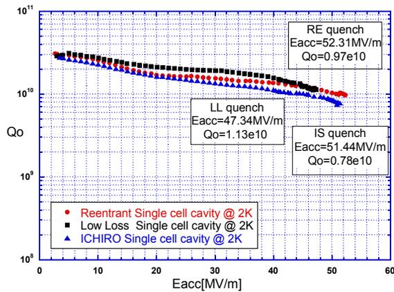
Figure 2: RF test results of the single-cells with different shapes, from Ref. [2].
