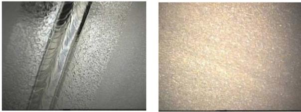
Figure 12: Picture of the inner surface of the equatorial EBW before (left) and after (right) removing 60  $\mu\text{m}$  by CBP.
