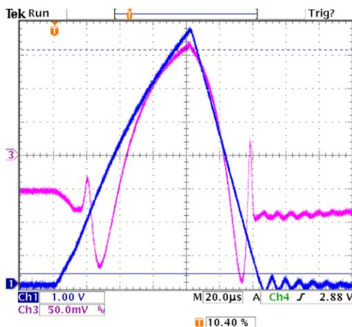
Figure 6: Type III fast phase shift (CH3 @  $\sim 17^\circ/\text{div}$ ) and solenoid bias current (CH1 @ 50A/div) as a function of time (20 $\mu\text{s}/\text{div}$ ).
