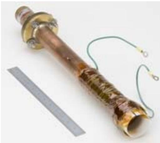
Figure 5: Type III phase shifter (slotted) with solenoid used for low power fast response tests.
