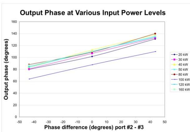
Figure 8: Vector modulator output phase as a function of phase shift difference.
