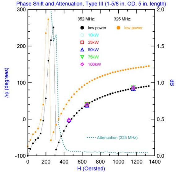
Figure 2: Type III phase shift and attenuation.
