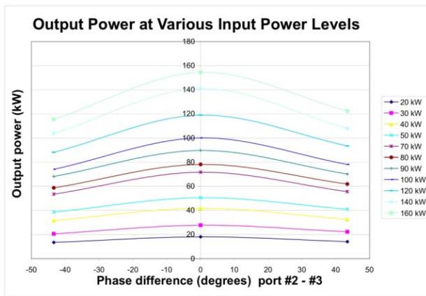
Figure 7: Vector modulator output power as a function of phase shift difference.
