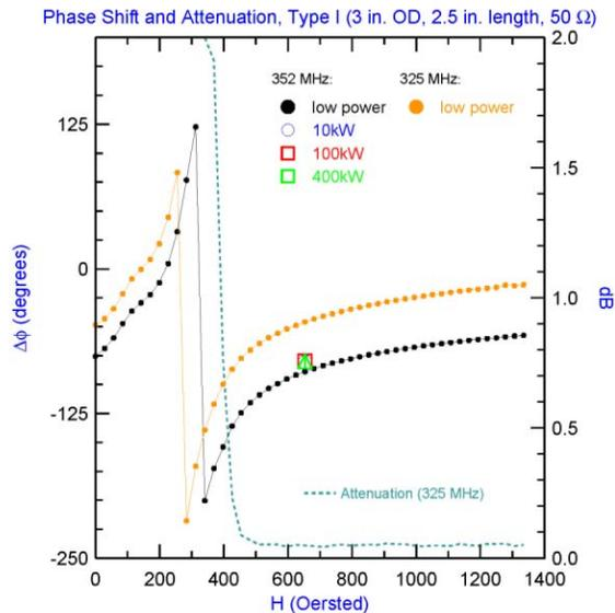
Figure 4: Type I phase shift and attenuation.
