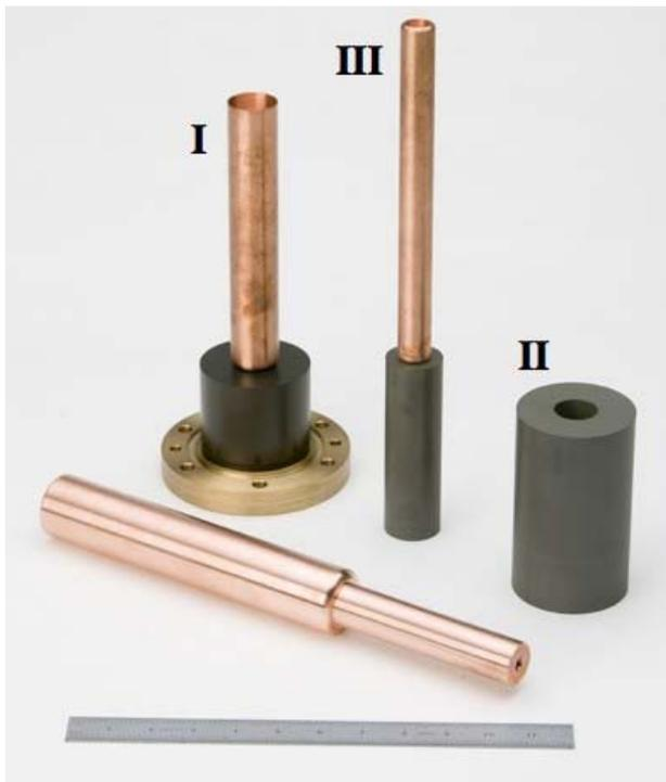
Figure 1: Components of the three types of phase shifters with a 12" ruler for scale.
