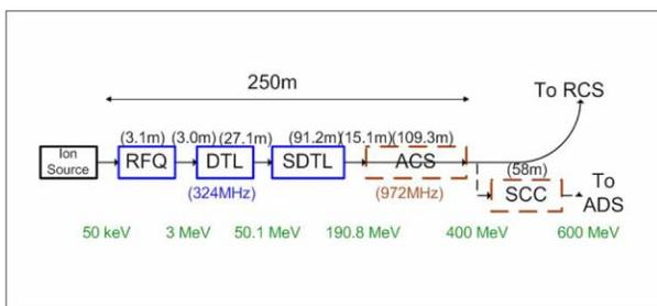
Figure 3: Scheme of J-PARC Linac
