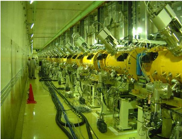
Figure 4: The SDTL's installed.
