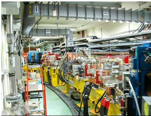
Figure 6: Injection region of Delay Loop with the waveguides feeding the 1.5 GHz RF deflectors
