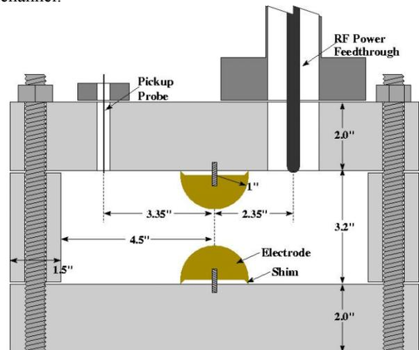
Figure 1: Cross section of the test cell showing the replaceable one inch radius Cu, Mo, or Be hemispherical electrodes. The top and bottom plates and the cylinder are copper-plated stainless steel (the gas input/exhaust port is not shown in the figure).
