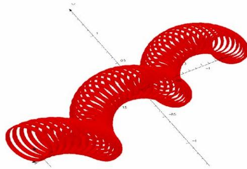
Figure 4: A new solution to the Helical Cooling Channel to be used in the 6D cooling demonstration experiment is made up of a series of superconducting coils which are displaced from each other as shown in the figure to create solenoidal, helical dipole, and helical quadrupole fields. At the beginning of the cooling channel, the 50 cm diameter coils produce about 5.5 T of solenoidal field.
