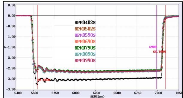
Figure 4: Calibrated BPM beam current signals up to module 10. The BPM0402 signal is acquired in front, all the others after the magnetic chicane.
