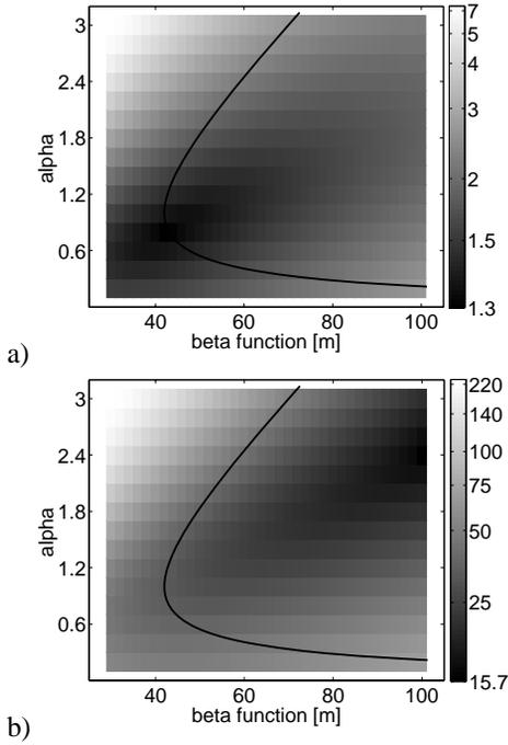
Figure 2: Dependence of ISR (a) and CSR (b) emittance growth on initial beta function and alpha. White means low emittance growth and black means high emittance growth. The black lines mark the initial values giving a symmetric beta function.
