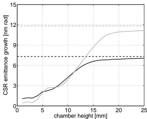
Figure 5: CSR emittance growth vs. chamber height (solid) in the C-chicane (solid gray) and the S-chicane (solid black). For comparison the free space CSR emittance growth is also plotted (dashed)
