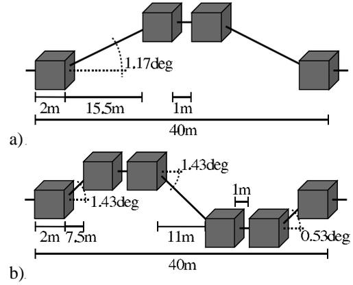
Figure 3: Optimized geometries of the C-chicane (a) and the S-chicane (b).
