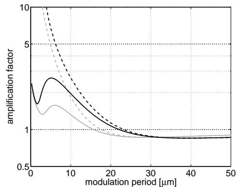
Figure 6: Gain of an initial density modulation due to the CSR microbunch instability in the C-chicane (gray) and the S-chicane (black) with  $\sigma_{E,\text{unc}} = 0$  eV and  $\varepsilon_{n,x} = 0$  nm rad (dashed) and  $\varepsilon_{n,x} = 570$  nm rad (solid).
