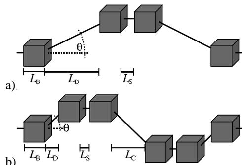
Figure 1: C-chicane (a) and S-chicane (b).
