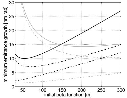
Figure 4: Minimum ISR (dashed), CSR (dash dotted) and ISR+CSR (solid) emittance growth vs. dipole shift for the C-chicane (gray) and the S-chicane (black).
