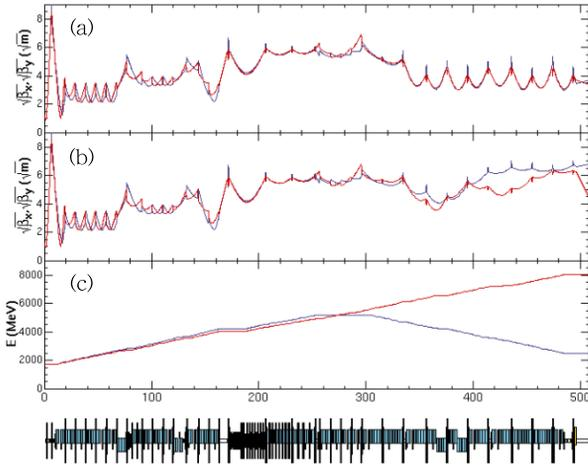
Figure 2: Optics between sector C and 5 for 2.5 GeV(a) and 8 GeV(b). Blue line shows horizontal and red line shows vertical beta functions. Beam energy is shown in the bottom.
