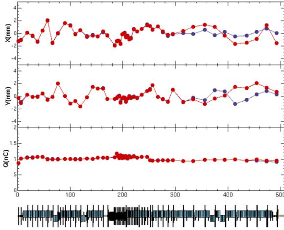
Figure 3: Orbits and beam charge per pulse between sector C and 5. Blue line shows 2.5 GeV and red line shows 8 GeV electron beam.
