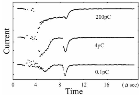
Figure 6: Change of pulse shape by changing the beam intensity
