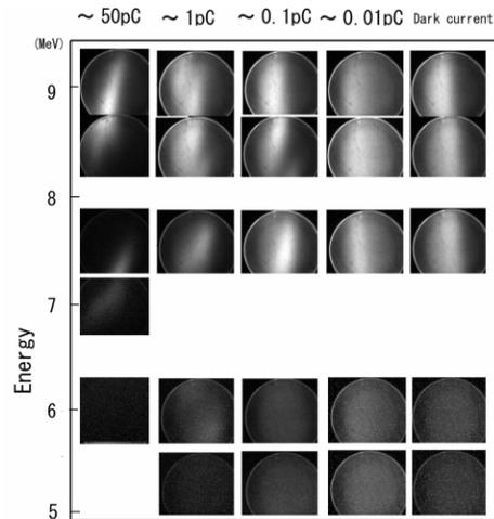
Figure 5: Brightness distribution of low intensity beam profile corresponding to the energy spectrum.
