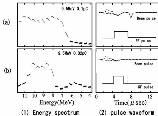
Figure 7: Change of pulse shape and the energy spectrum by changing the pulse width of RF pulse.
