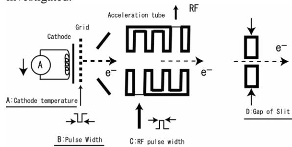
Figure 1: Modulation methods for beam weakening.
