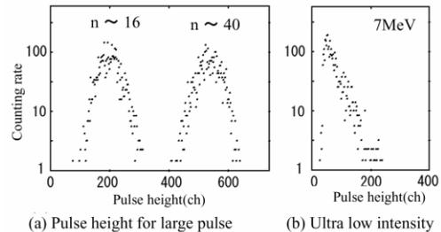
Figure 4: Pulse height distribution of NaI(Tl)scintillator for low intensity electron beam.
