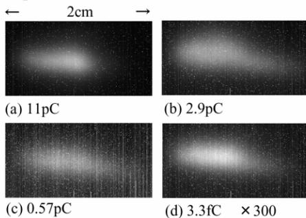
Figure 3: Beam profiles obtained by the cooled CCD system.
