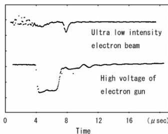
Figure 8: Pulse shape of ultra low intensity electron beam and the high voltage of the electron gun.
