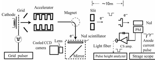
Figure 2: Layout of ultra low intensity beam experiments.
