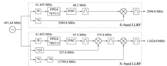
Fig 3: Single station RF controller block diagram.
