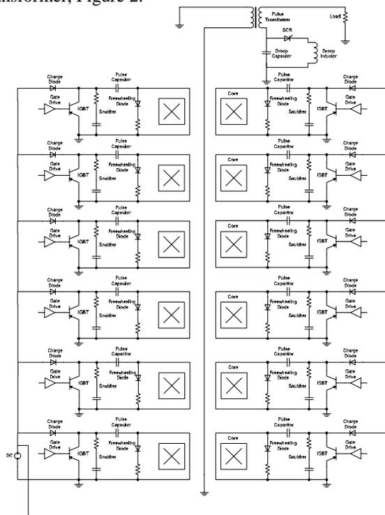
Figure 2: Solid state modulator layout.
