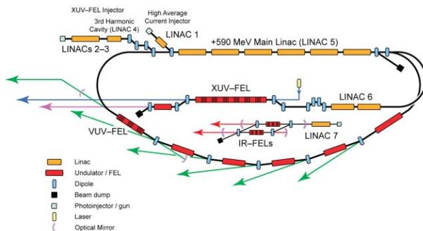
Figure 1: 4GLS Conceptual Layout and SRF Linacs.
