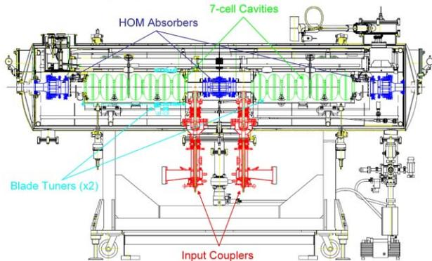
Figure 7: Modified Stanford Cavity/Cryomodule.
