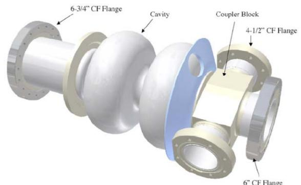
Figure 2: Cornell 2-Cell CW Injector Cavity Design.
