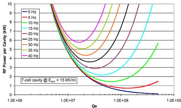
Figure 5: Microphonics Impact on  $Q_e$  and RF Power.
