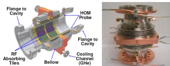
Figure 6: Cornell ERL Injector HOM Absorber.
