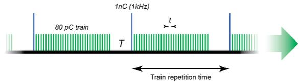
Figure 4: Possible Bunch Structure for 4GLS.
