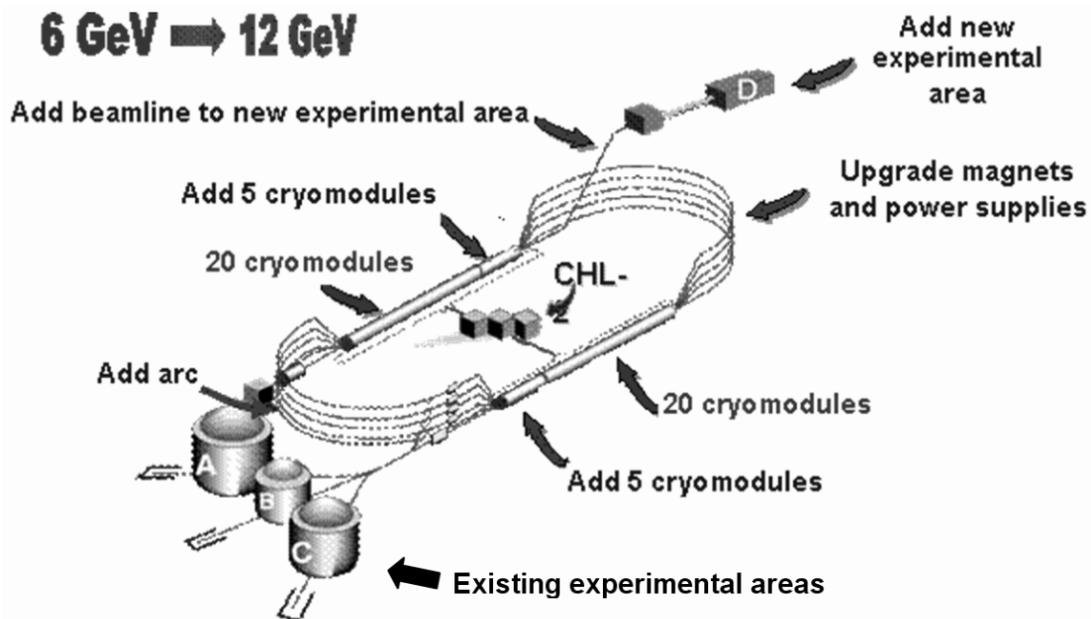
Figure 1: Conceptual illustration of upgrading CEBAF to 12 GeV.
