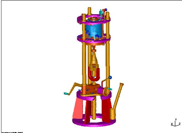
Figure 3: The tuning installation with the gun cavity.
