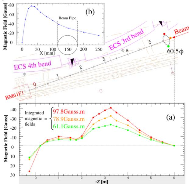
Figure 2: Measurements of magnetic leak from ECS.
