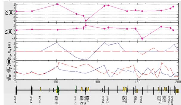
Figure 5: Measured dispersion functions after setting the correction factors in Table 1 to the quads.
