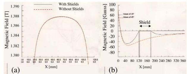
Figure 3: Calculations of magnetic fields of the ECS bend.
