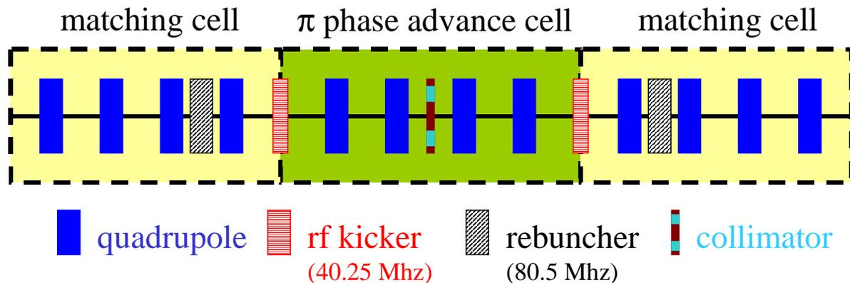
Figure 1: Layout of the front-end MEBT with the beam distribution system hardware for the RIA driver linac.
