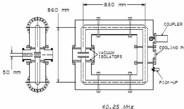
Figure 4: 40.25 MHz HW resonators for the kickers of the RIA MEBT beam distribution system.
