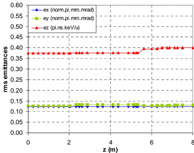
Figure 3: Beam rms emittances along MEBT.
