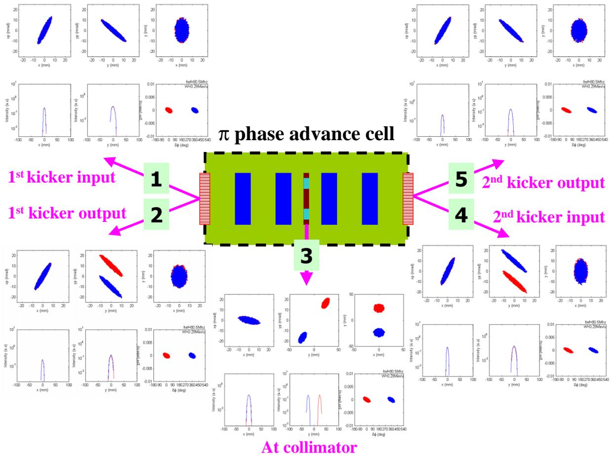
Figure 2: Motion of two consecutive 80.5 MHz bunches (red/light, blue/dark) along the  $\pi$  phase advance cell for ideal fields in the 40.25 MHz rf kickers. For each location, top row pictures are  $xx'$ ,  $yy'$  and  $xy$  spaces, bottom row pictures are horizontal profile, vertical profile and  $\delta\phi\delta W$  phase space. At the third location, the scale of the  $x$  and  $y$  axes were changed for display.
