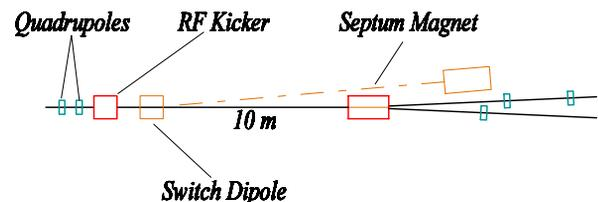
Figure 6: BSY beam distribution system layout.
