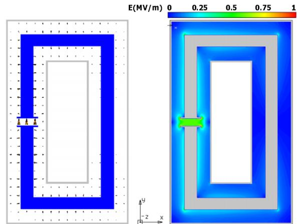
Figure 5: Deflecting field in the MEBT rf kickers.
