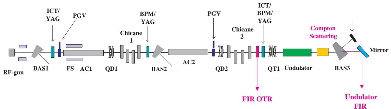
Figure 4: Layout of FIR linac. (QD: quadrupole doublet, FS: focusing solenoid, AC: accelerating column, QT: quadrupole triplet, BAS: Beam energy analyzer, and YAG: YAG screen).
