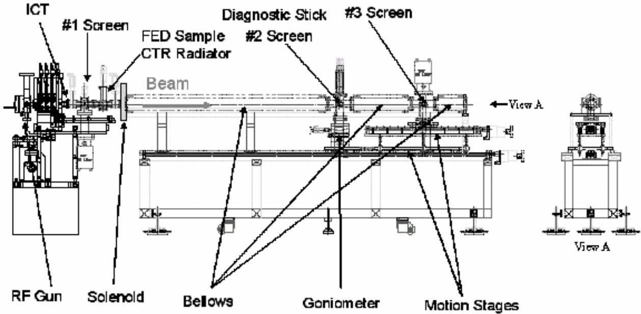
Figure 1: Schematic diagram of experimental setup of the gun test stand for fs-FIR facility.
