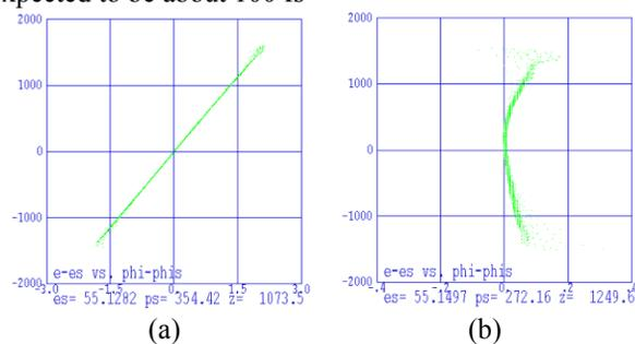
Figure 5: PARMELA simulation for bunch compression by Chicane-2 from (b) to (a).  $es$ : the synchronous particle energy,  $phis$ : the synchronous particle phase. The vertical axis is  $e - es$  in MeV and the horizontal axis is  $phi - phis$  in degrees. One degree corresponds to about 1ps.
