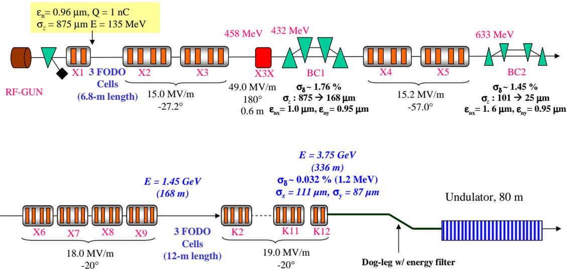
Figure 1: Layout of the PAL-XFEL injector and linac.
