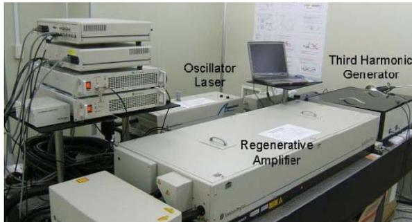
Figure 3: A picture of Ti:sapphire system.
