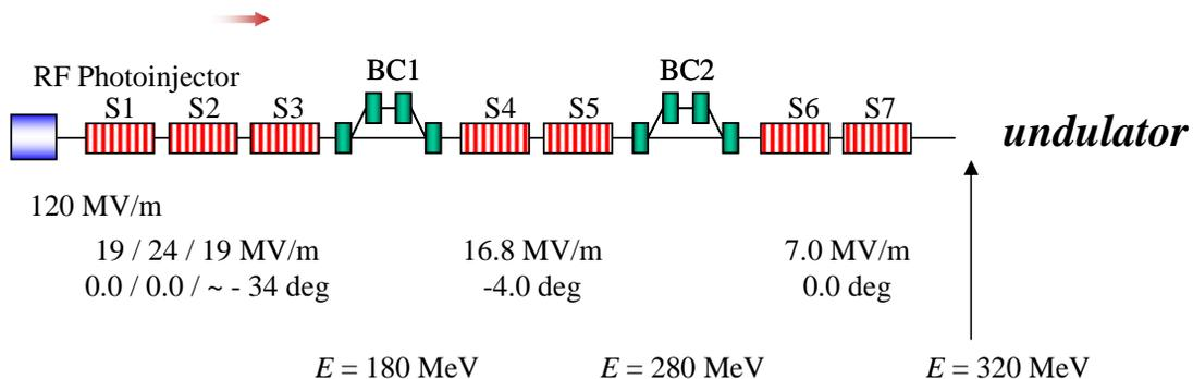
Figure 2: Layout of the test linac.
