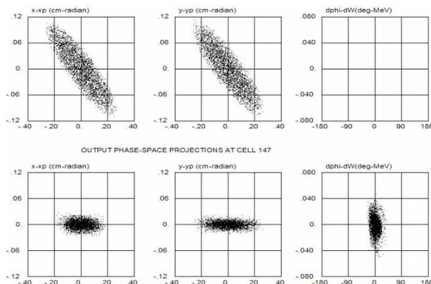
Figure 6: Phase Space Projections In and Out of RFQ.
