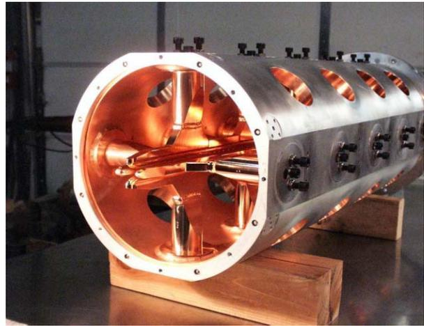
Figure 3: Radial-Strut, Four-Bar RFQ.
