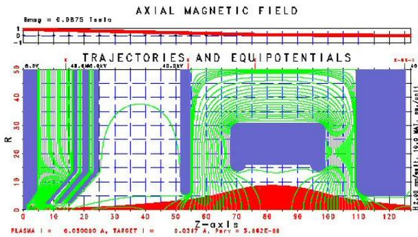
Figure 2: Beam Profile from Ion Source through LEBT.
