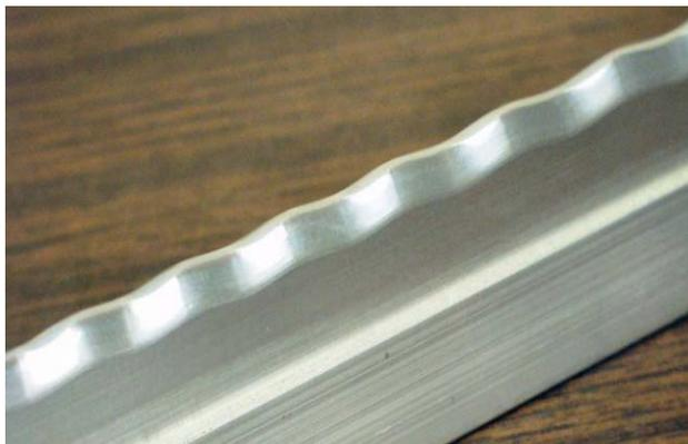
Figure 7: Surface of an existing RFQ Bar as machined.
