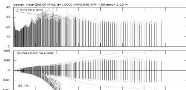
Figure 5: Radial and Energy Profiles through RFQ.
