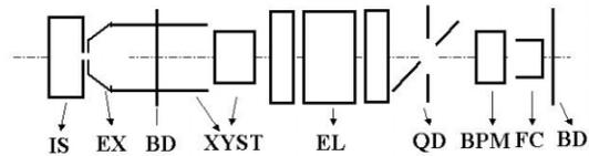
Figure 2: ECR ion source and LEBT (IS: ion source; EX: Extraction; BD:Beam diaphragm; XYST: X and Y steer; EL: Einzel lens; QD: Quadruple diaphragm; BPM: Beam position monitor; FC: Faraday cup).
