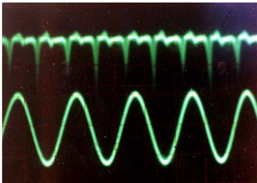
Figure 10: Simultaneous accelerated  $O^+$  and  $O^-$  beam in 1MeV ISR RFQ-1000.
