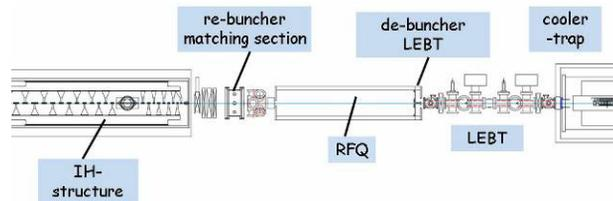
Figure 2: Overview of the RFQ section of the HITRAP decelerator.
