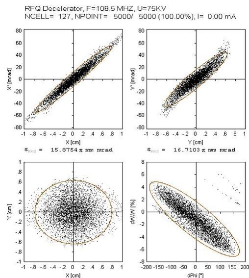
Figure 6: Output distribution with deactivated Debuncher.
