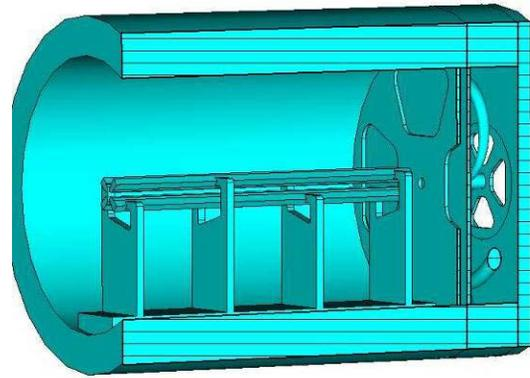
Figure 4: Low energy section of the RFQ and the Debuncher cavity.
