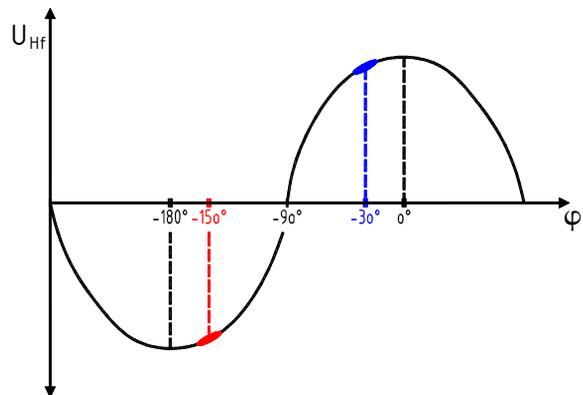
Figure 3: synchronous phases of a bunch leaving the accelerating structure and of a bunch that is injected into a decelerator.
